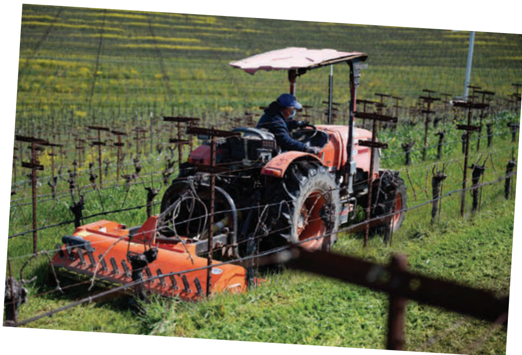
Flail mowing in East Hill Gewürztraminer vineyard. The vine prunings are placed in the middle of the rows and this flail mower chops them into little pieces. Later in the spring the chopped biomass is incorporated into the soil, helping reduce Navarro's carbon footprint.
