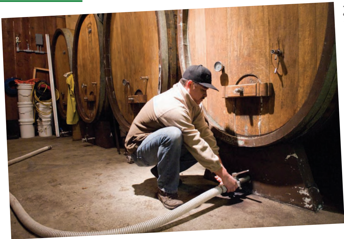
Alfredo hooking up a hose to an older oval with an oak door. (Our newest ovals have stainless steel doors.) Since we aren't trying to add oak flavors, the primary purpose of these casks is to let the wine age and clarify on the yeasts produced during fermentation. The ovals in the photo are about 50 years old. Hugel Winery in Alsace uses an oak oval, Sainte Catherine, that dates back to 1715.
