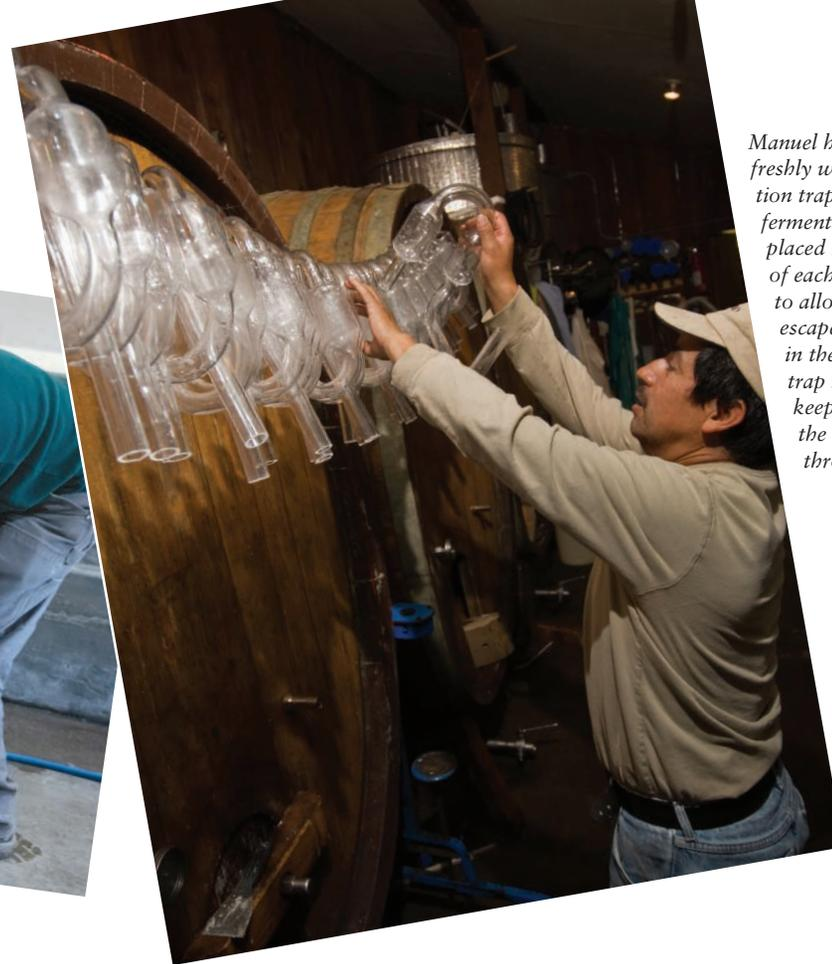
Manuel hanging up a freshly washed fermentation trap to dry. During fermentation a trap is placed in the bunghole of each large oak oval to allow the CO<sub>2</sub> to escape. The cylinder in the middle of the trap holds water to keep flies out but the CO<sub>2</sub> bubbles through the water.
