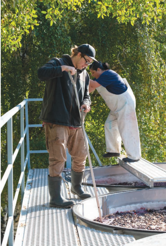
Punching down Zinfandel in an open-top fermenter is a twice-daily chore. We have ten open-top fermenters which are used to ferment Zinfandel, Syrah, Grenache Noir, Sangiovese and Carignane.
