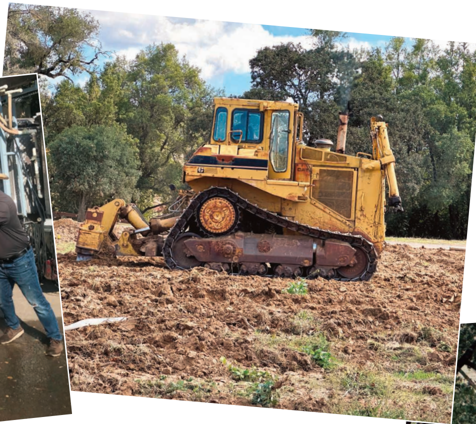
These are the three-foot shanks that the Cat is using to rip through the soil.
