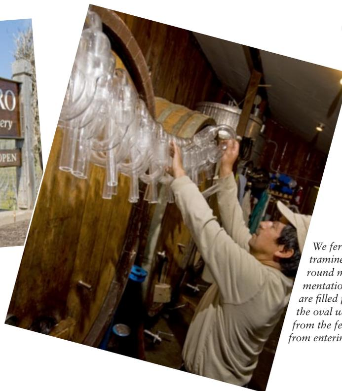
We ferment all our Pinot Gris and Gewürztraminer in French oak casks to generate a round mouth-feel. Manuel is cleaning the fermentation locks for these large casks. The locks are filled partially with water and inserted into the oval which allows carbon dioxide to escape from the fermenting wine, yet keeps the oxygen from entering.
